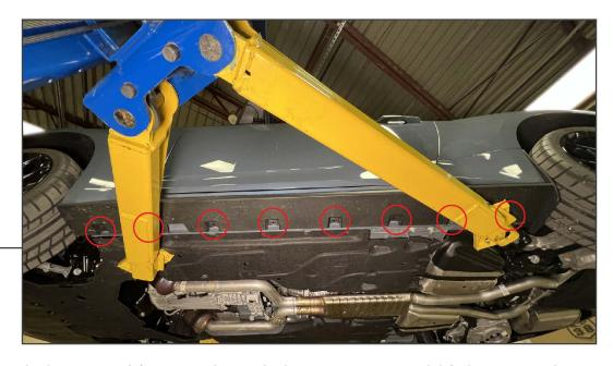
From under the vehicle, remove (8) rectangular push clips. Using a pry tool, lift the rectangular clip towards the ground to release the clip.
