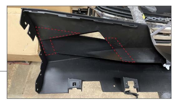
Test fit the included grille panel to the side skirt, and familiarize the flat portion of the grille fitment in relation to the side skirt. Once familiar with fitment, apply the included adhesion promoter to the grille flat panels and the side skirt.
