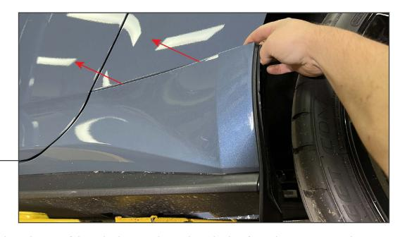
Firmly pull back on the top of the side skirt to release the side skirt from the quarter panel.
