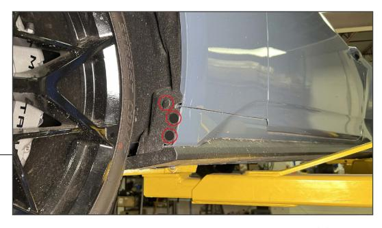
Safely lift and support the vehicle off the ground. Inside the front wheel well, remove (3) plastic push clips from the fender liner/side skirt.
