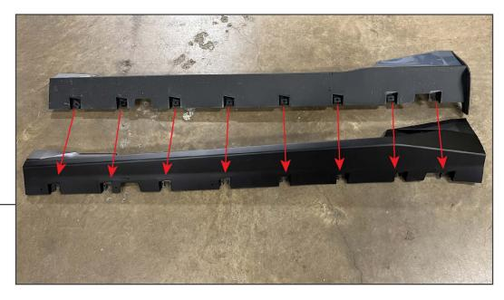
Place the new side skirt and the original side skirt on a soft workable surface.
