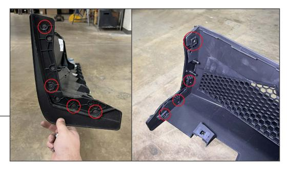
Remove (4) T-15 Torx screws from the OEM mud guard on the side skirt. With the mud guard removed, remove the screw retainers from the side skirt.
