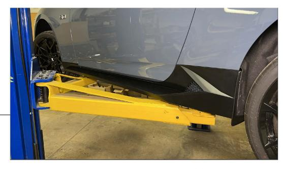
Secure the bottom of the side skirt to the vehicle rocker panels using the (8) original rectangular push clips. Secure the fender liners to the vehicle reusing the original hardware.
