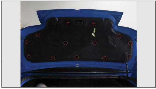
Remove the (13) plastic clips holding the trunk liner to the trunk lid. Once loose, remove the trunk liner and set aside.
