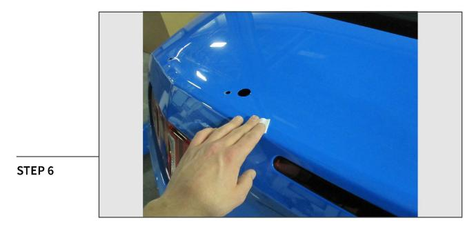
Once the trunk lid is free of adhesive, wipe down any areas where the new spoiler's tape will adhere with the supplied Alcohol Prep Pads.
