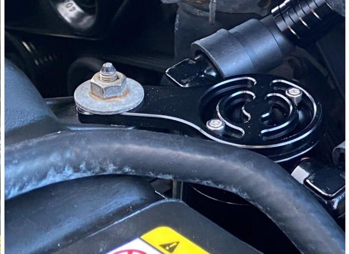
1. Remove the factory nut on the coolant bottle tank. Install the UPR catch can bracket onto the stud and reinstall the nut.
