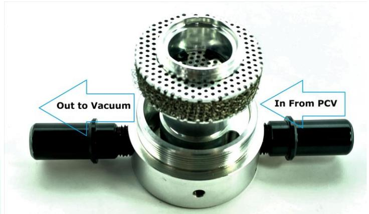
3. The catch can outlet will be marked with a silver ring at the end of the fitting. This is the outlet side to the vacuum source. The other side is the inlet from the PCV.
