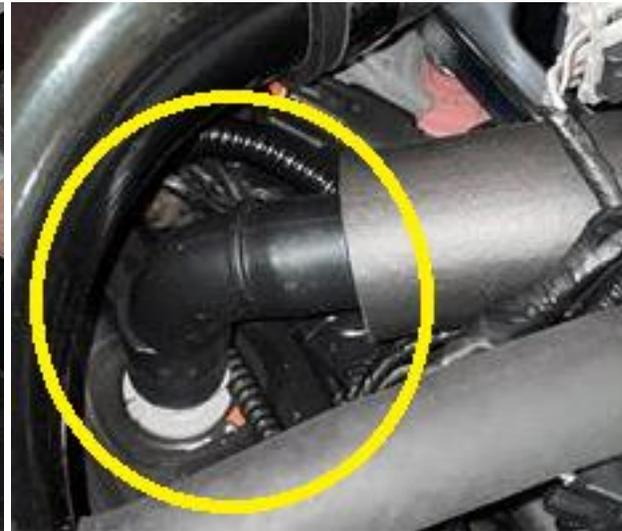
2. Locate and remove the factory PCV hose. It will run from the vacuum fitting on the front side of the throttle body to the PCV fitting on the passenger side valve cover.
