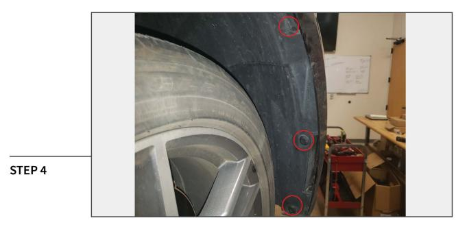
On each side of the bumper, remove the plastic clips holding the fender liner to the bumper.
