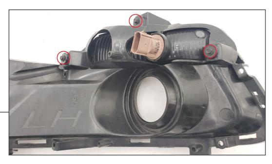
Remove the (3) 7mm screws securing the factory turn signal light to the fog light bezel. Remove the turn signal light.
