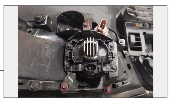
Remove (3) 7mm screws securing the fog light to the fog light bezel. Remove the fog light from the bezel.
