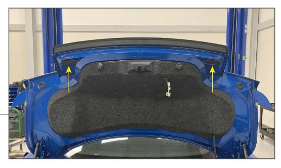
Open the vehicle trunk. Remove the (2) plastic covers from each end of the trunk lid behind the decklid panel.
