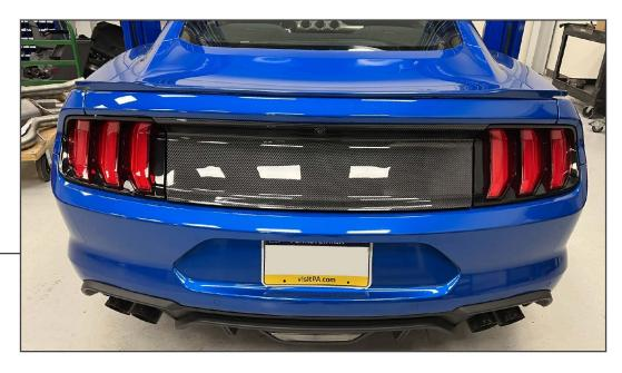
Align the decklid panel to the vehicle, and plug the rear camera harness into the camera assembly. Press the new decklid panel into the vehicle trunk lid, and secure into place using the original hardware. Re-install the OEM trunk lid plastic covers over the hardware holes.
