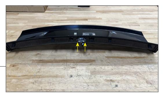
Remove (2) 7/32" screws from the rear camera assembly. Transfer the camera to the new decklid panel reusing the original screws.
