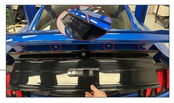
Using a plastic pry tool, firmly pry the decklid panel downwards to disengage the (4) metal retaining clips. Transfer the clips to the new decklid panel.
