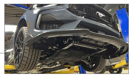
Fit the LH side and RH side chin spoiler panels into the vehicle bumper. Press firmly to engage the plastic retaining tabs into the vehicle bumper.
