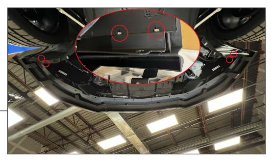
Secure the outer edge of the LH and RH chin spoiler panels to the bumper edge using (2) Phillips bolts and (2) M6 nuts per side.
