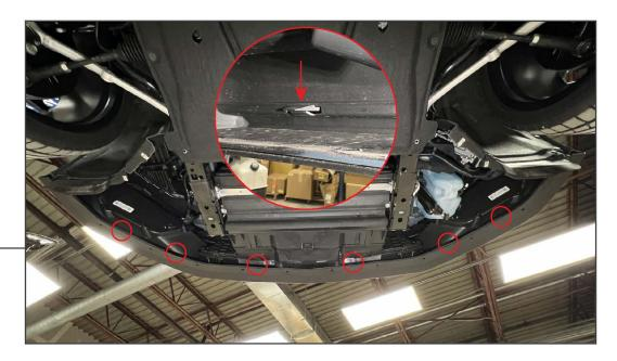
Begin removing the chin spoiler from the bumper by working from the outside of the vehicle towards the middle. Using a metal pry tool, press down on the chin spoiler retaining tabs while gently pulling the chin spoiler away from the bumper.
