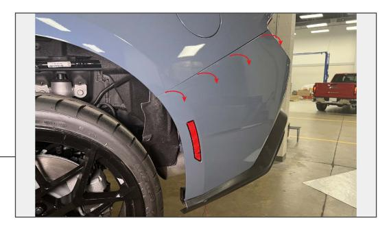
Firmly pull the edge of the bumper away from the vehicle quarter panel. Use of a plastic panel tool may be necessary to dislodge the retaining clips/adhesive.
