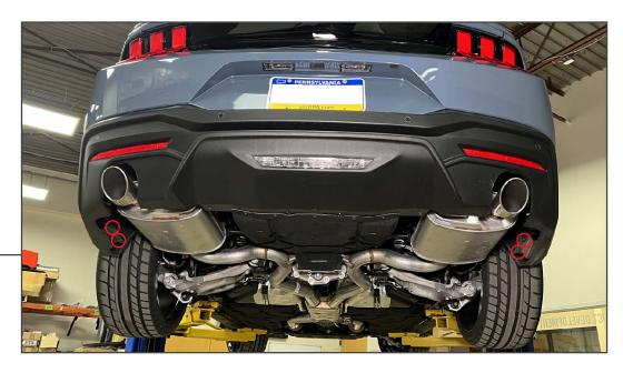
Safely lift and support the rear of the vehicle above the ground using a floor jack and jack stands. From under the vehicle, remove (2) plastic push clips from each side of the bumper.
