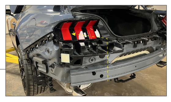
With assistance, begin to lift the rear bumper and diffuser to the vehicle. Route the red & blue wires towards the vehicle LH tail light through a suitable vehicle trunk grommet. Splice the wires into the vehicle following the diagram below.
