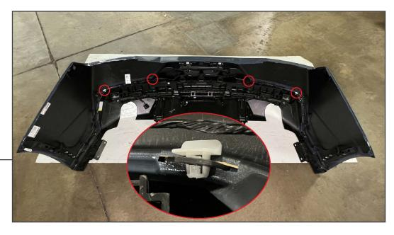
Remove the (4) plastic clips joining the diffuser to the bumper by pressing the plastic tab and lifting the clip out.
