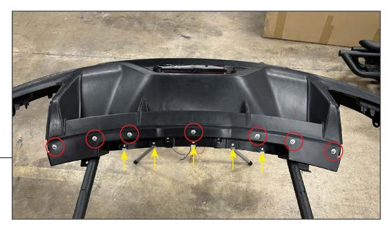
Secure the lower diffuser panel to the diffuser using (7) Phillips bolts, (7) flat washers, and (7) clip nuts. Tighten evenly until secure.
