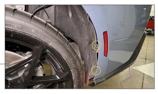
Remove (1) plastic push clip and (2) 7mm screw from each rear fender liner. Manipulate the liner from the vehicle bumper to access the bumper hardware.
