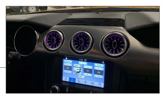
To change airflow, twist the center of the air vent 90 degrees to open/close the air vent.
