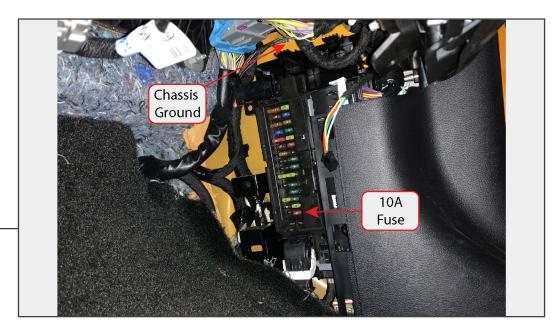
Remove the trim panel covering the vehicle fuse box. Locate and remove the 10A fuse at the bottom of the fuse box. Connect the RED wire on the RGB module to the included fuse tap. Fit the 10A fuse into the fuse tap along with the included fuse. Install the fuse tap into the 10A fuse slot.
