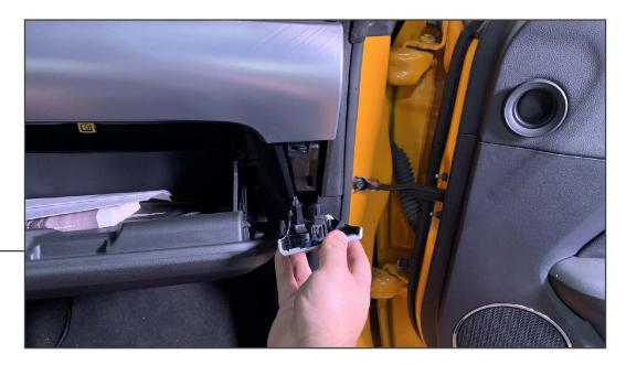
From the passenger side of the vehicle, use a plastic trim removal tool to remove the lower trim panel from the vehicle dashboard. Lower the glove compartment for additional working space. Rock the panel back-and-forth while pulling away from the dashboard to dislodge the clips if necessary.
