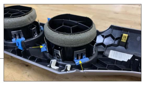
Using a small flathead screwdriver, gently pry the (4) plastic tabs on the OEM air vents, and push the vents through the face of the dashboard panel.
