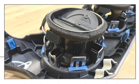
Press the LED harness into each air vent housing. The connector will snap into place when secure.
