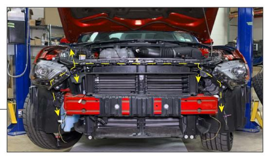
Neatly route the included wiring harness along the vehicle core support. Route the light connectors on each side of the shutter assembly. Then, route the Yellow wire leads to each vehicle turn signal/fog light connector. Route the Red/Black wire leads towards the vehicle fuse box/battery.
