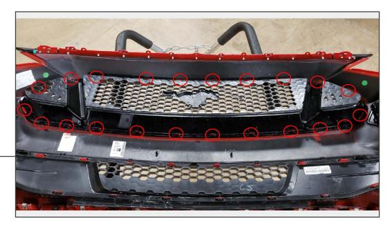
Remove the factory upper grille by manipulating the tabs with a flathead screwdriver. Then, remove the upper grille and set aside.
