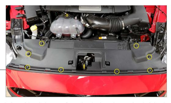
Lift and support the front of the vehicle using a floor jack and jack stands. Open the vehicle hood.
