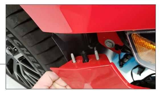
Carefully use firm pressure pull the edge of the bumper down to pop it from the clip. With assistance, support both sides of the bumper and slowly remove the bumper and support it on a soft, non-abrasive surface.
