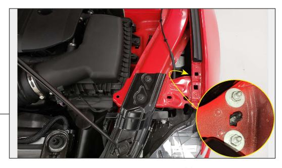
From the top between the fender on each side, locate and remove the (2) 10mm nuts securing the bumper to the fender, then remove the bracket.
