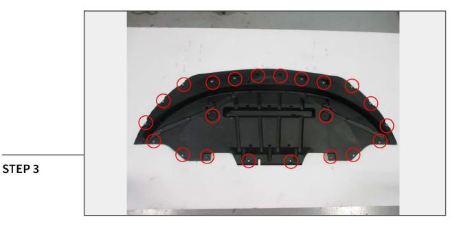
Support the front of the vehicle to can access the bumper splash shield. Remove the mounting hardware to disconnect the splash shield from the vehicle.
