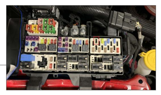
Crimp the included fuse tap to the Red wire on the harness. Fit the fuse tap into the fuse indicated below, neatly route the harness out of the fuse box and close the lid. The lights will power on with key on ignition.
