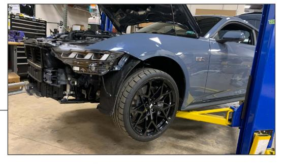
Raise the vehicle so that the tires are just off the ground. Support the vehicle with jack stands. Using a lug wrench, remove the wheel.
