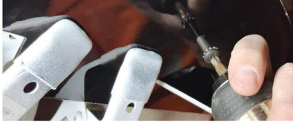
16. Hand tighten all side blade mounting screws. Be sure to not over tighten and strip out side rocker plastic. Repeat full side blade process for other side blade.
