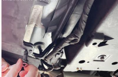
For added security after installing silver screws, add silver screw on washers to silver screws
