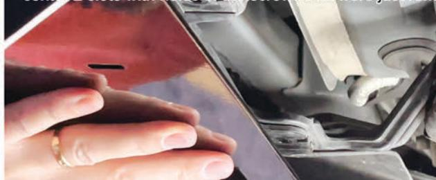
10. Use silver screws with small lock washers to mount center diffuser section. Pinch the middle of the stock diffuser and EMP diffuser together to get screws in further and ensure it is secure before letting go. Place a pad on ground underneath just in case.
