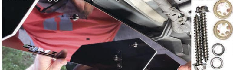
11. Diffuser is slotted so you can adjust how far out you want the diffuser. Once diffuser is in place, tighten silver screws with 1/4" wrench and ensure diffuser remains straight and at the distance from the car you desire.
