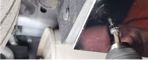
15. Double-check that side blade is still in the position you desire, then install screw closest to tire, then rear screw and lastly the center screw.
