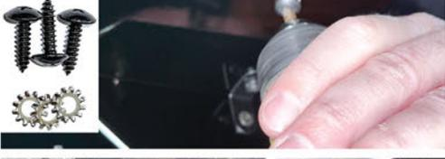
NOTE: For 2015-17 model add a screw in the center hole under reverse light (optional on 2018+ due to larger gap). Do not over tighten screws. You could strip out the plastic in the stock diffuser. If this happens, obtain a larger #12 stainless steel screw.
