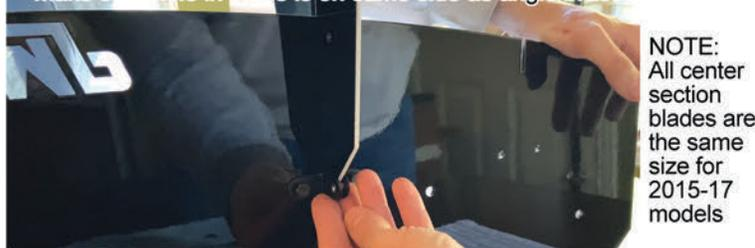
5. Insert 3/4" screw from side shown then place lock washer on screw then hex nut. Fully tighten this screw with 1/8" bit and 3/8" wrench. Check that blade is straight then tighten other 2 screws.
