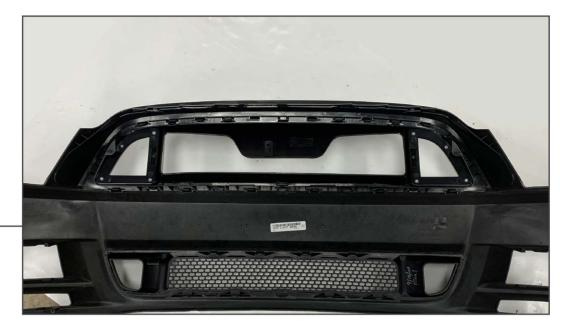
Press the new grille into the vehicle through the front, and ensure all the perimeter mounting clips are securely pressed into place.
