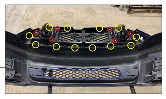
Place the bumper on a soft workable surface. Remove the OEM fog lights by removing (3) 7mm screws per light assembly.
