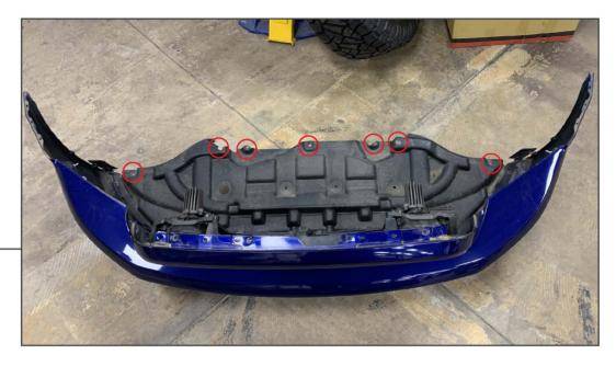
From under the vehicle, remove (7) 7mm bolts from the rear of the splash shield.
