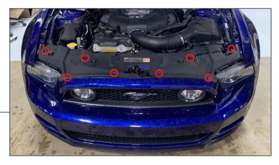
Open the hood. Remove the (8) plastic push clips from the radiator support cover. Remove the cover from the vehicle.
