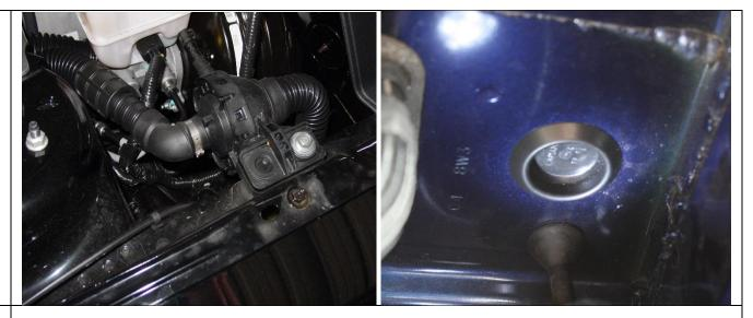
Plug in MAF sensor and supplied PCV hose (hose can be shortened to your liking depending on how you route it) Use light oil in helping slide hose onto fitting on bottom of tube.
