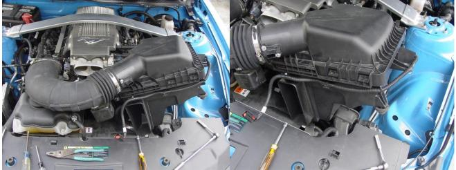
5 Remove front air inlet coming from the grille. Use flat screwdriver to undo the 4 tabs (1 on each side). Once you get 2 or more give it a good tug straight out and it will pop off.
