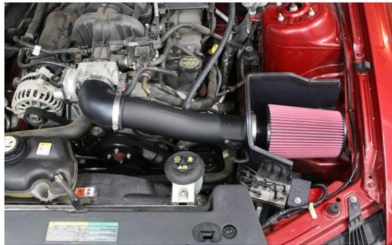
**Oil Filter:** The frequency you should clean your filter will depend on your driving conditions. It is recommended to check your filter at every oil change or 3,000 miles. If there is a buildup of dirt as thick as the wire mesh, then it's time to clean your filter. To properly clean your oil filter, we recommend the S&B Precision Cleaning & Oiling Kit (located in the Parts Sold Separately Section of our website, [www.JLTtruecoldair.com](http://www.JLTtruecoldair.com)).
