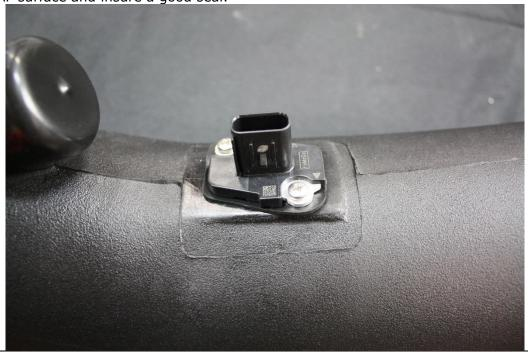
**AUTOMATIC CARS ONLY:** Drill a 1/2" hole above the PCV grommet, insert Automatic grommet and fitting. See picture below.
