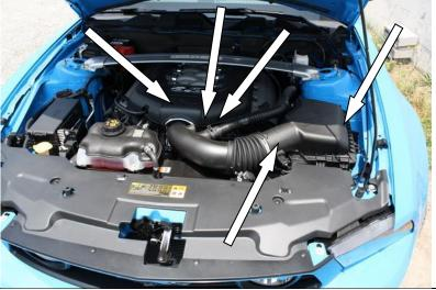
Remove rubber mounting grommet and metal insert from stock air box and install in JLT Heat Shield. Set JLT shield into stock location, squeeze rubber air inlet and insert into shield and bolt down using stock air box bolt.
