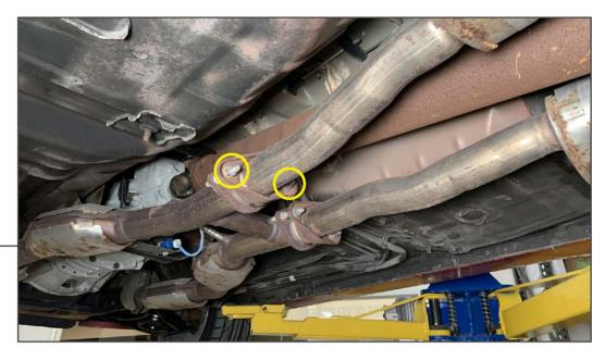
Safely lift and support the vehicle off of the ground using a floor jack and jack stands. Remove the (2) 9/16" nuts from the front exhaust flange.
