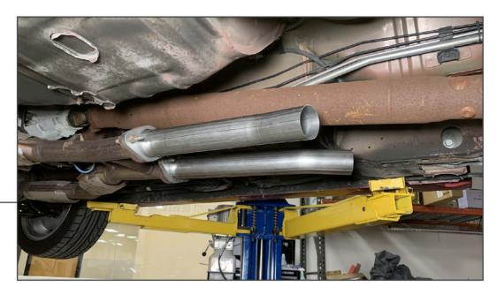
Identify the included front pipes. The longer front pipe fits onto the RH (Passenger) side of the exhaust. Fit (1) exhaust flange onto the front pipe, and loosely secure to the vehicle exhaust using the original (2) 9/16" nuts. \*\*The flanges are directional, ensure the tapered inner portion faces the original vehicle exhaust pipes to ensure a proper seal.
