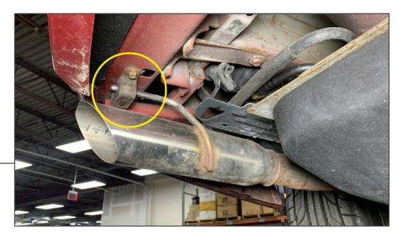
Locate the exhaust hanger behind the rear bumper. Slide the exhaust assembly from the hanger, and remove the exhaust from the vehicle. Repeat steps 1-3 for the remaining exhaust assembly.
