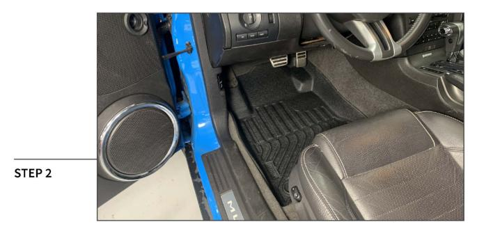
Align the floor liner to the vehicle floor and press into place. If applicable, align the floor liner into the vehicle floor retaining studs.
