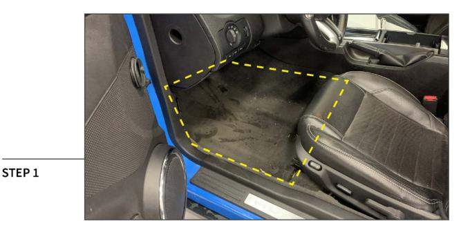
Remove any existing floor mat from the vehicle. Clean the vehicle carpet using a vacuum cleaner.
