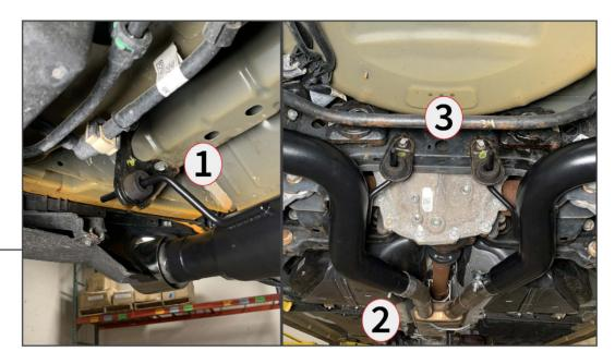
Insert the rear of the new muffler pipe into the rear most hanger (1). Then, slip the muffler pipe into the cut vehicle resonator pipe fully (2). Bolt the rear subframe exhaust hangers to the rear subframe using the original bolts (3).
