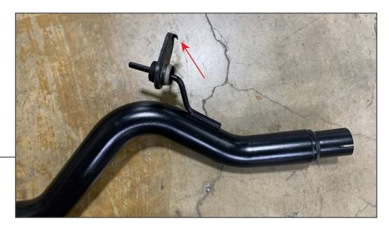
Transfer the rear subframe exhaust hangers from Step 2 to the new exhaust pipes. Ensure the metal hook faces towards the inlet of the exhaust pipe.
