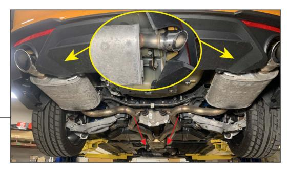
Push the entire exhaust system towards the rear of the vehicle within the hangers above the mufflers. Remove the front pipe from the resonator, then lower the front of the exhaust. Slide the rear section of the exhaust from the upper hangers, and remove the exhaust from the vehicle.
