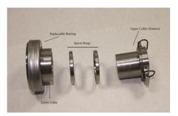
To remove the ring(s), pull the upper collar with one hand and the bearing and lower collar with the other hand. Twist the collars as you pull on them and they will separate the components. The upper collar has an O-Ring on the ID to retain the lower collar. The spacer rings just slip off of the lower collar. If the collars are dry, the resistance during disassembly will require greater effort to separate the components, continue to pull and they will separate.
