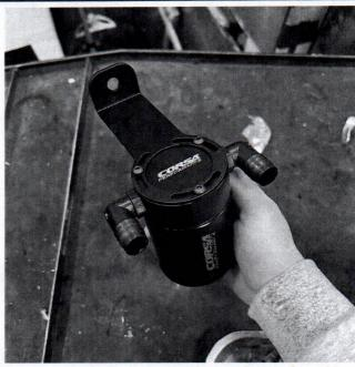
1. Locate your vehicle's PCV line and remove it. Find a mounting location for your Corsa Catch Can. Use the provided bracket(s), fittings, and hose to route the catch can to the PCV system. The A end of the catch can is the inlet, the B end of the catch can is the outlet. IMPORTANT: Corsa Performance highly recommends applying PTFE tape or thread sealant to the fittings and the bottom drain plug to avoid any leaks.
