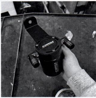
1. Locate your vehicle's PCV line and remove it. Find a mounting location for your Corsa Catch Can. Use the provided bracket(s), fittings, and hose to route the catch can to the PCV system. The A end of the catch can is the inlet, the B end of the catch can is the outlet. IMPORTANT: Corsa Performance highly recommends applying PTFE tape or thread sealant to the fittings and the bottom drain plug to avoid any leaks.
