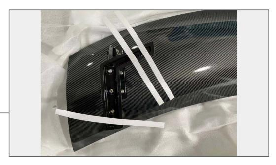
Using the included drilling template strips, align each strip to the threaded holes in base of the assembly. Once adhered to the spoiler, peel the tape backing and place the spoiler to the vehicle trunk lid and allow adhesion to the vehicle. Remove the spoiler, and drill the mounting holes using a 17/64" drill bit.
