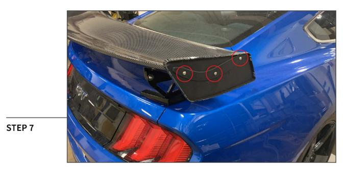
Install the spoiler inner end caps using (3) M6 x 15mm Allen bolts. Tighten until secure.
