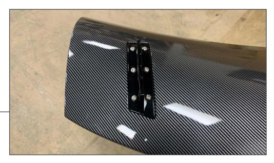
Place the spoiler on a soft surface. Install brackets labeled "3" using (6) M6 x 12mm Allen bolts per bracket. Tighten until the brackets are secure.
