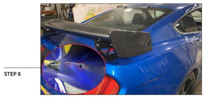
Place the spoiler outer end caps onto the inner end cap, the outer clips will audibly click into place when secure. Secure the outer end cap using (2) Phillips head screws through the inner end cap.
