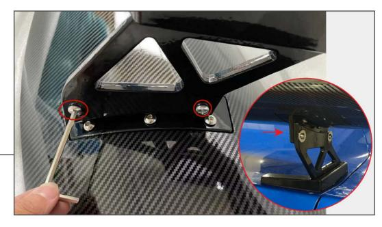
Secure the assembled "1" and "2" brackets to the spoiler bracket "3" using (2) M6 x 25mm Allen bolts, (4) M6 flat washers, and (2) M6 nuts per side.
