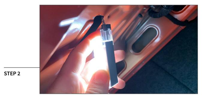
Unplug the factory light and install the LED light in reverse order. Installation is now complete.
