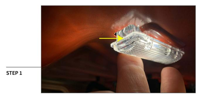
Using a thin plastic pry tool, depress the light's locking tab and pull the light down and away from the vehicle.
