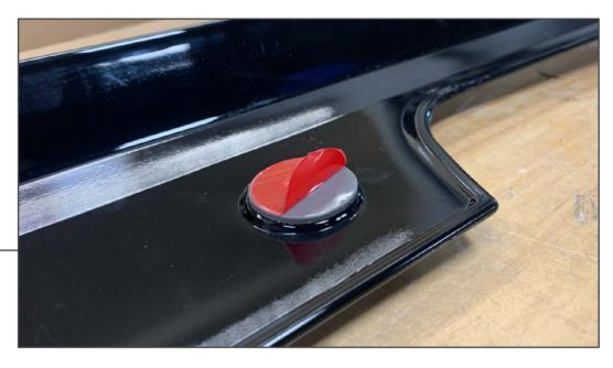
Become familiar with the fitment of the wicker bill to the spoiler. Center the wicker bill to the spoiler, while allowing the wicker bill to sit flush against the rear of the spoiler. Peel back the tape backing from the (4) circular tape pads and adhere the wicker bill to the spoiler.
