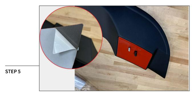
Ensure the outer mounting surfaces are clean and dry. Peel back the white tape backing and install the die cut tape pad to the spoiler.
