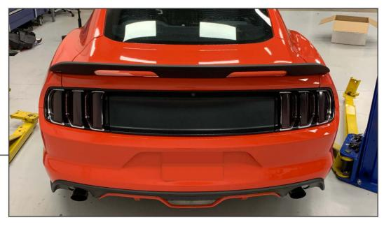
Peel back the red tape backing on the spoiler tape mounting pads. With a helper, install the spoiler to the vehicle using the (4) flanged nuts. Once installed, apply pressure over the taped surfaces to ensure proper adhesion.
