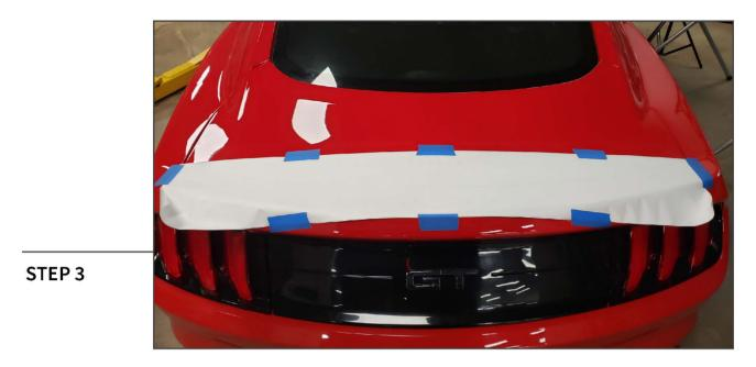
Using the supplied template, align the edge of the template with the edge of the trunk lid. Use masking tape to secure the template to the decklid.
