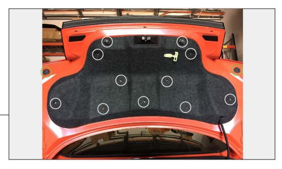
Remove the inner trunk panel by removing the (9) plastic push rivets, (2) rubber bumpers, and the plastic trim around the latch assembly. There are also (2) rubber plugs on the far left and right of the trunk lid that will need to be removed to gain access to the factory bolt locations. If your vehicle came equipped with a factory spoiler, carefully remove it using adhesive remover and a soft pry tool.
