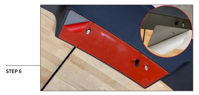
Ensure the middle mounting surface is clean and dry. Peel back the white tape backing and install the die cut tape pad to the spoiler.
