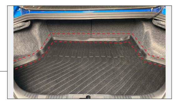
Place the cargo liner into the vehicle cargo area. Ensure the front and side edges of the cargo liner are raised to allow the liner to fully fit into the cargo area.
