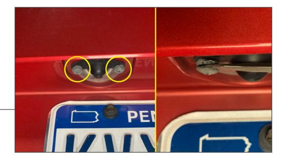
Remove the (2) plastic clips using a Phillips screwdriver.
