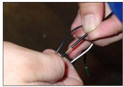
Splice the black wire to the black to ground out the HALO. Wrap the electrical tape around the two splicers.
