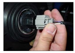
Pull the headlight housing straight out and disconnect the harness from the headlight bulb.
