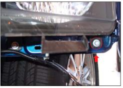
Remove the two 10 mm screws located at the bottom the headlight housing.
