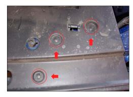
Remove the 3 push pins on the passenger side from the radiator shroud.
