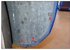
Remove the three phillips screws that hold the fender shroud to the bumper.
