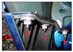
Remove the 10 mm nuts that hold the bumper to the fender.
