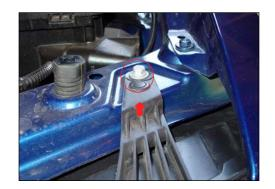
Remove the 10 mm screw located on the top of the headlight. Also remove the push pin located in front of the screw.
