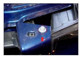
Remove the 10 mm screw from the top of the bumper located next to the headlight. Remove bumper by pulling straight out.
