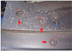
Remove the 3 (three) push pins on the driver side from the radiator shroud.
