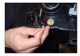
On the Anzo USA™ headlight assembly the HALO will have exposed plugs, cut the plugs off.
