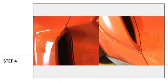
Test fit the part before removing the tape backing. The top edge of the scoop sits on the edge of the body line radius. The opening should sit about 1/16"-1/8" off the edge of the door opening. Remove the tape backing, align the scoop, and apply firm pressure to all the tape surfaces to fully seat the adhesive.
