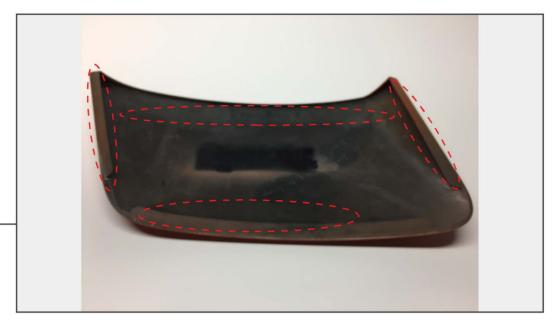
Thoroughly clean your vehicle using automotive soap and water. Using the supplied alcohol pads, clean the tape ledges. Once the alcohol is dry, wipe the tape ledges with the supplied adhesion promoter, allow to dry.
