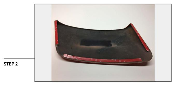
Trim and install the supplied tape to the treated tape ledge surfaces. Note: If you did not order the Side Scoop Inserts, skip to Step 4.
