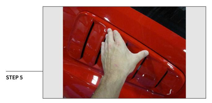
Once the louver is properly positioned around the quarter window, firmly press down around the entire edge of the louver to fully seat the adhesive.
