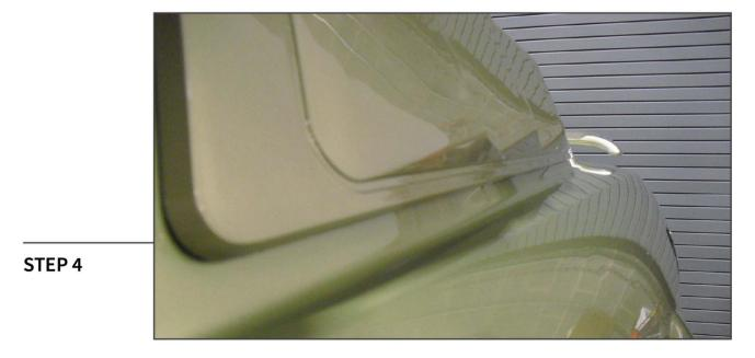
Lightly place louver on vehicle in desired location, making sure the bottom edge is parallel to the body line as shown in picture.
