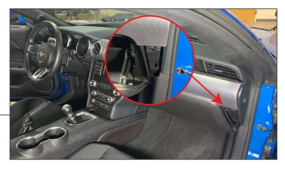
Using a soft pry tool, remove the plastic trim to the right of the glove box.
