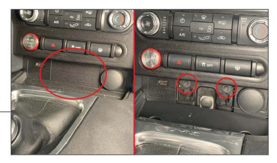
Using a flat blade screwdriver, pry the plastic rectangle from the dashboard. Remove the (2) 7mm screws securing the bottom of the radio to the vehicle.
