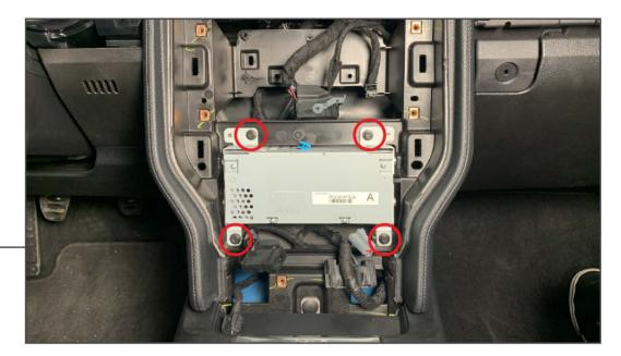
Remove the (4) 7mm screws from the radio module. Disconnect the (3) electrical connectors from behind the module. Remove the module from the vehicle.
