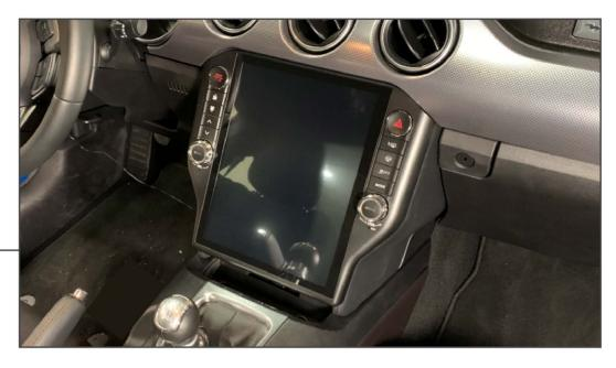
Transfer the yellow/orange panel clips from the factory dash panel onto the new display. Then, install the navigation head unit into the vehicle re-using (4) 7mm screws. Re-assemble the vehicle following steps 1-4 in reverse order.
