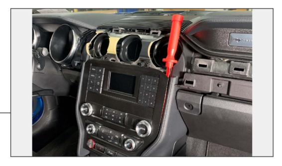
Using a panel removal tool, stick the tool down the side of the radio. Pry on the tool while pulling the radio to release the clips securing the radio to the vehicle. Repeat the procedure to the opposite side of the radio.
