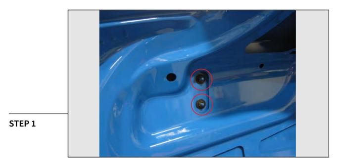
Open the trunk lid and remove the four 10mm nuts securing the factory spoiler to the trunk lid. BE SURE TO HAVE SOMEONE HOLDING THE SPOILER SO IT DOES NOT DROP AND HIT THE VEHICLE ONCE THE NUTS ARE REMOVED.
