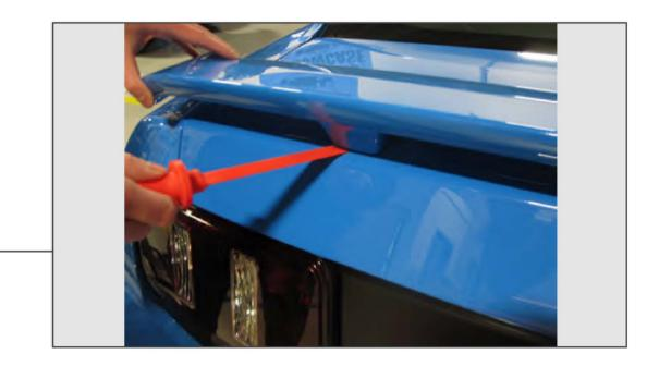
Close the lid and use a plastic pry tool that will not scratch your paint and remove the spoiler from the decklid. Do not pry against the decklid, it will dent/crease. Only use pry tool to gently wedge between the spoiler and decklid surface. Once the spoiler is removed, use adhesive remover to clean up any residue left by the factory adhesive tape. A heat gun or hair dryer can help soften the tape and make removal easier. Overheating the surface can cause paint damage, use minimal heat.
