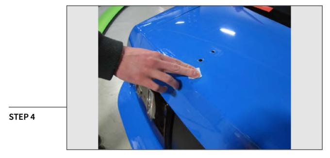
Wipe down the decklid surface with the supplied alcohol prep pads as shown. Be sure to wipe all areas that the adhesive on the new spoiler will come in contact with.
