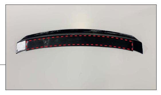
Using the provided roll of double sided tape, adhere the tape to the designated area of the spoiler. Clean the spoiler using (1) alcohol prep pad. Once dry, adhere the tape to the spoiler.
