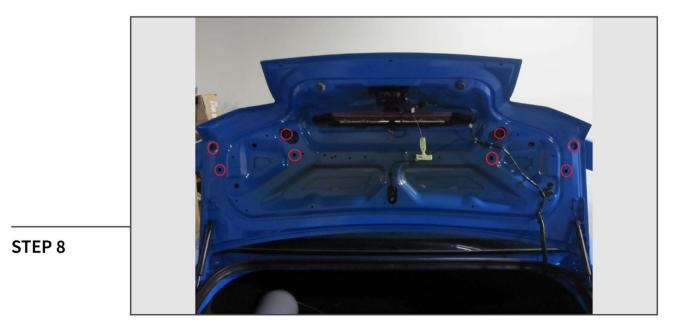
Remove the double sided tape backing from the (4) pedestal pads. With assistance, install the spoiler using the (8) supplied M6 screws. Once fully tightened, reinstall the trunk liner removed in Step 1.
