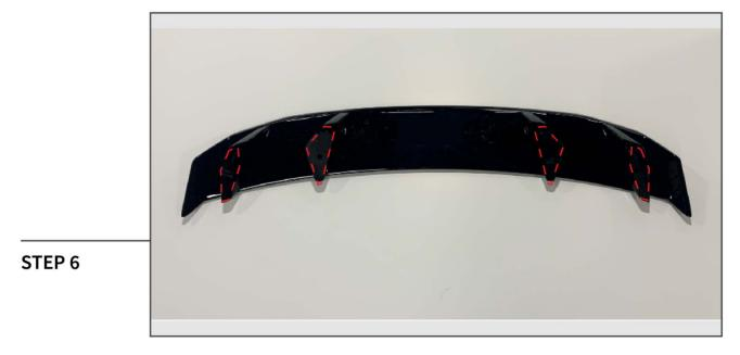
Lay the new spoiler on a soft flat surface and place the included double sided tape pads on the four pedestals as shown.
