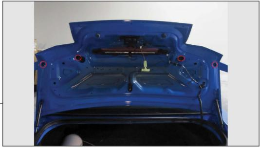
Use a 10mm socket to remove the (4) nuts holding the factory spoiler to the vehicle.
