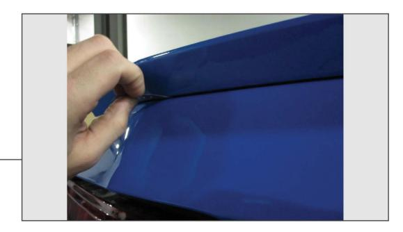
Use a heat gun around the edges of the factory spoiler to loosen the adhesive. It may also help to gently pry the spoiler up and run around the edges with a razor blade as shown. Once the adhesive is loose, remove the factory spoiler form the vehicle. **DO NOT OVERHEAT THE PAINT, DAMAGE MAY OCCUR.**
