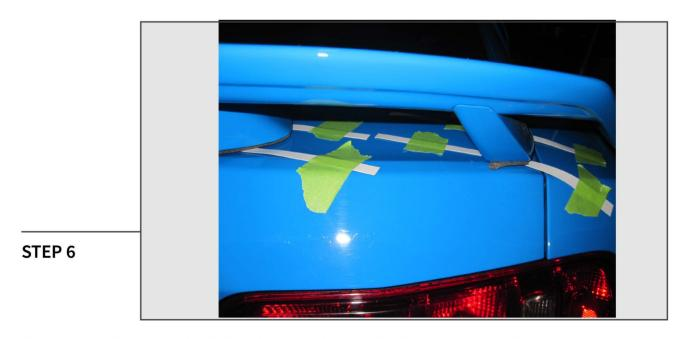
Place the spoiler on the decklid, making sure to align the four rearward holes on the new spoiler with the factory holes in the decklid. Once properly located, use masking tape to tape the template strips to the decklid as shown.
