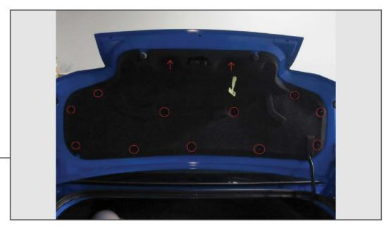
Remove the 13 plastic clips holding the trunk liner to the truck lid. Simply pull outward on them and they will pop out. Once loose, remove the trunk liner.
