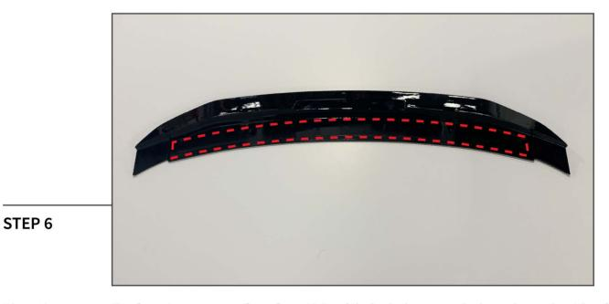
Place the new spoiler face down on a soft surface. Using (1) alcohol prep pad, clean the underside of the spoiler where the spoiler will adhere the trunk lid. Once dry, place and adhere the provided double sided tape to the perimeter of the spoiler mounting area.
