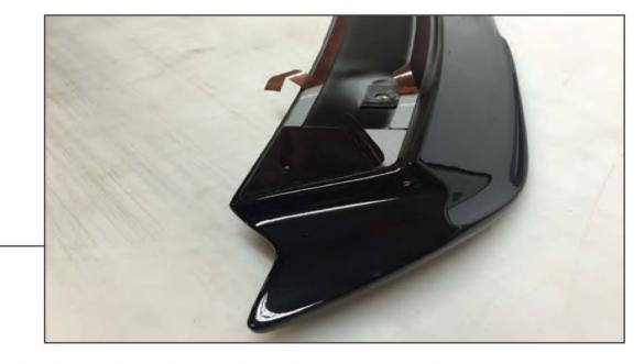
Place the supplied foam pads over the mounting holes on the spoiler, trim as needed.
