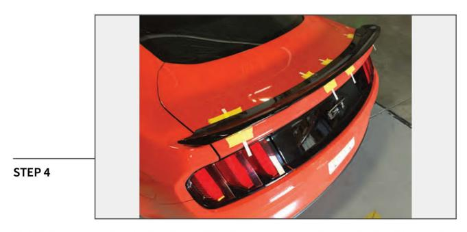
Test fit the spoiler and center it on the decklid. Then tape the templates to the decklid where they lay. Carefully remove the spoiler from the templates. This step is extremely import and will determine the final fitment of the spoiler. Please take your time and ensure the spoiler is seated properly before taping down the drill templates to the decklid.
