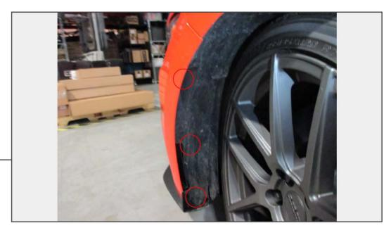
On each side of the bumper, remove the plastic clips holding the wheel well liner to the bumper/splash shield.
