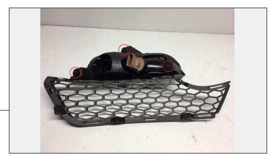
Install the factory turn signals onto the new turn signal bracket using the factory screws. Then install the new bracket onto the bumper using the factory hardware.
