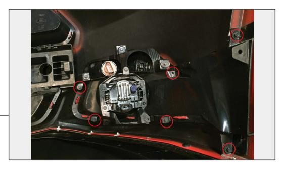
Using a 7mm socket, remove the screws holding the turn signal bracket to the bumper. Use a flat head screwdriver to assist in releasing the clips.
