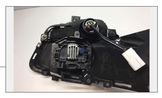
Using the existing hardware, reinstall the Smoked LED Turn Signal.
