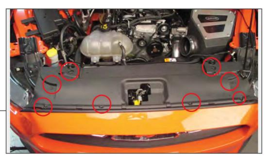
Remove the (8) clips securing the plastic radiator cover to the radiator support and remove the cover from the vehicle.
