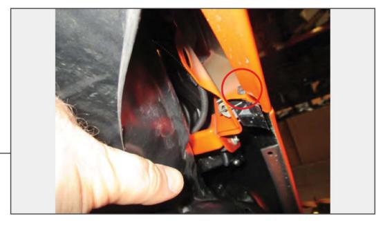
Fold back the fender liner so that you can access the one bolt that holds the bumper to the fender. Once removed, firmly pull the sides of the bumper away from the fender.
