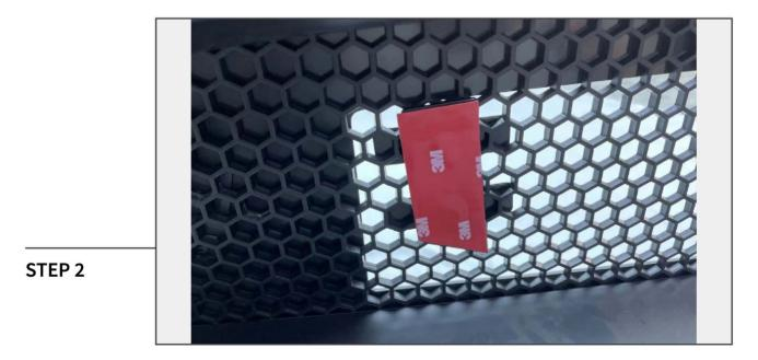
Clean the metal emblem holder using isopropyl alcohol and a microfiber cloth. Once dry, adhere the supplied double sided tape to the metal emblem holder. Apply firm and even pressure to ensure the tape is fully adhered to the emblem holder.
