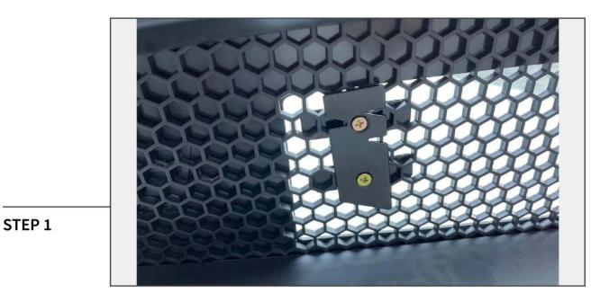
Place the metal emblem holder in a suitable location of the grille facing outward. Using (2) threaded spacers on the inside of the grille and (2) Phillips screws, secure the base to the grille.
