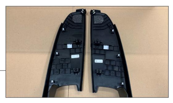
Cut out the drilling templates located at the end of the install guide. Place the templates in the designated location on both upper trim panels.
