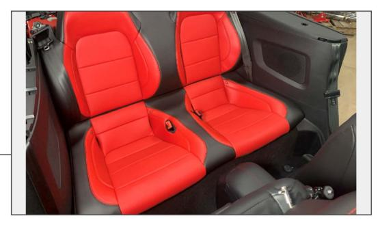
Install the rear seat cushion to the vehicle. Be sure the seat belt buckles are in their appropriate locations.
