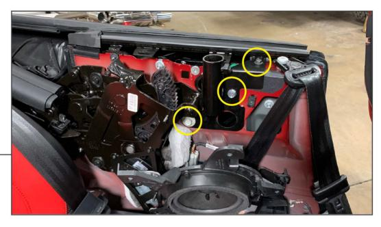
Install the labeled styling bar brackets to the vehicle. Reuse the (1) 15mm window motor assembly bolt and (1) 10mm rear window seal bolt. Install (1) 5/16-18 x 1" flange bolt and (1) 5/16 flange nut through the middle of the bracket to secure the bracket to the quarter panel. Leave bolts loose until all bolts are started. Tighten all bolts evenly.
