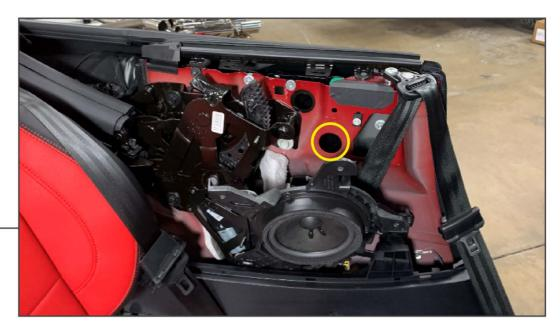
Remove the rubber grommet from the quarter panel using a panel removal tool.
