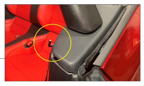
Apply pressure to the styling bar to ensure the styling bar fits evenly to the upper trim panel. Using a 6mm Allen Key, secure the styling bar to the brackets.
