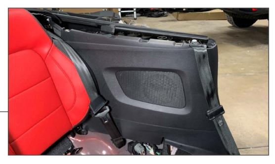
Reinstall the speaker cover panel to the vehicle.
