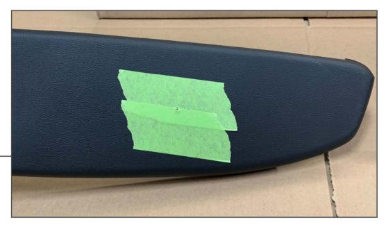
Place masking tape over the previously drilled hole. Using a 2" hole saw, drill a hole into the upper trim panel using the 1/8" hole as the guide hole. Once drilled, clean the hole of any remaining debris.
