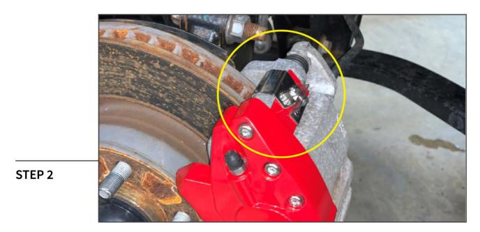
Align the upper caliper cover brackets to the top of the brake caliper bracket. Tighten the (1) Allen bolt and (1) 8mm nut using the provided tools to secure the caliper cover to the brake caliper.
