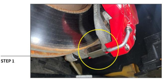
Safely lift and support the vehicle. Remove the front and rear wheels from the vehicle. Align the bottom of the caliper cover to the bottom of the brake caliper bracket.
