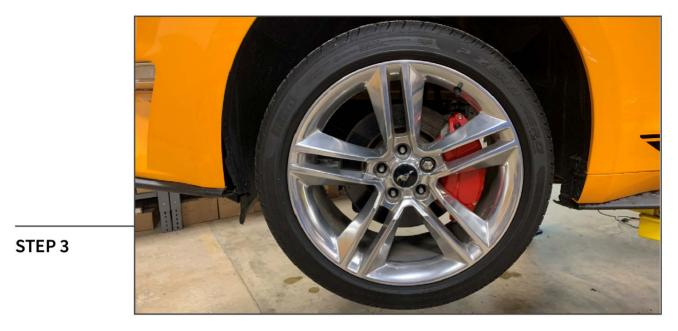
Re-install the wheels onto the vehicle. Safely lower the vehicle to the ground. See vehicle owners manual for proper lug nut torque procedure and specifications.
