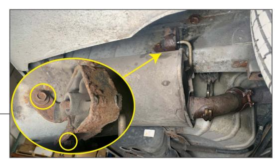
Remove (2) 13mm bolts from the exhaust hanger above the muffler.
