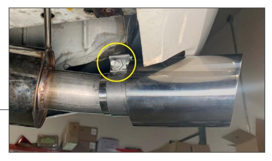
Slide the exhaust tip and (1) exhaust clamp onto the end of the muffler. Align the exhaust tip to the vehicle, then tighten the clamp.
