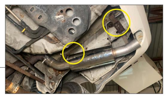
Slide the new muffler over the vehicle's exhaust pipe with the exhaust clamp on the muffler pipe. Install the (4) exhaust hanger bolts through the exhaust hangers to install the muffler to the vehicle.
