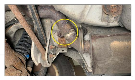
Safely lift and support the vehicle. Loosen the exhaust clamp at the back of the muffler.
