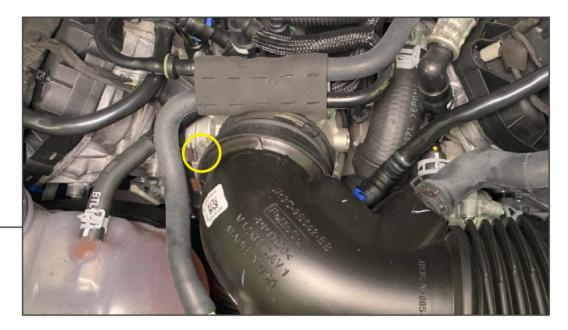
Loosen the hose clamp on the end of the intake tube attached to the throttle body.
