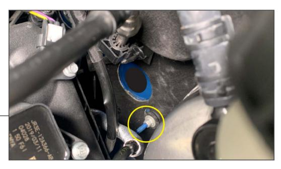
Remove the sound tube from the vehicle. Remove (1) 10mm nut from the firewall. Once removed, pull the sound tube away from the vehicle. Install the provided grommet into the firewall in place of the sound tube.
