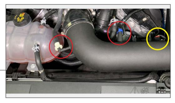
Install the PCV and vacuum lines to the intake. Push the lines onto each appropriate fitting until the clip clicks into place. Plug the MAF sensor harness into the MAF sensor.
