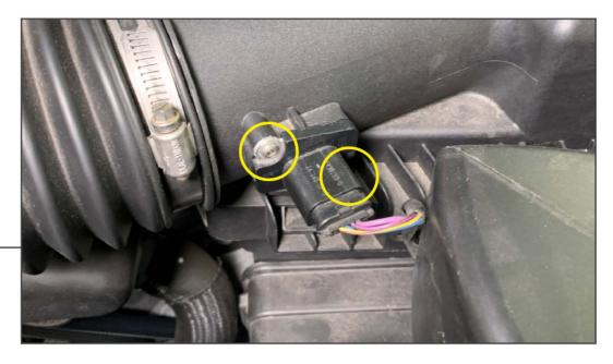
Remove (2) T-20 Torx screws to remove the MAF sensor from the intake tube.
