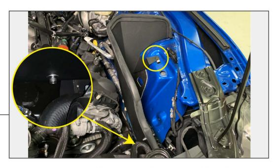
Install the weatherstrip along the top edge of the intake shield. Align the shield into the vehicle and install (1)  $M8x1.25 \times 15$ mm Allen bolt, (1) M8 lock washer, and (1) M8 flat washer to secure the bottom of the shield to the vehicle. Secure the top of the shield in the original bolt location reusing original hardware.
