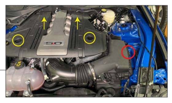
Remove the engine cover from the engine. Remove the (2) plastic covers on top of the cover using a flathead screwdriver. Remove the (2) 10mm nuts inside the cover. Firmly lift up on the cover, starting at the back, and remove the cover from the vehicle. Remove (1) 10mm bolt from the side of the air box.
