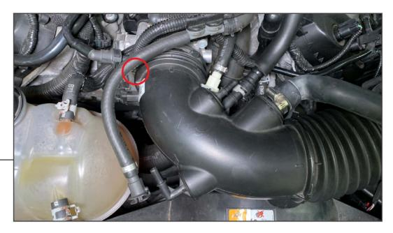
Loosen the hose clamp on the end of the intake tube attached to the throttle body.
