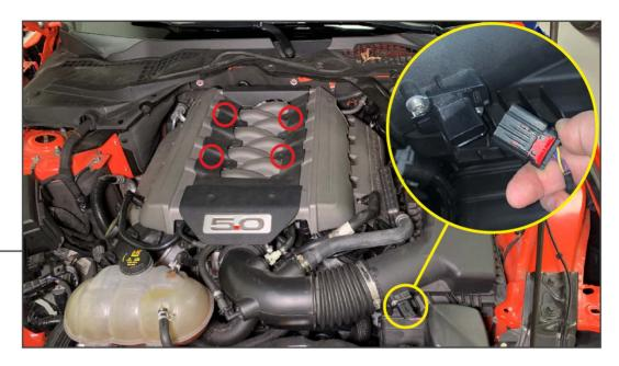
Remove the engine cover by firmly pulling up along the sides to release the cover from the (4) pins. Unplug the MAF sensor by sliding out the red lock, then pushing the connector tab in and pulling the connector away from the sensor.
