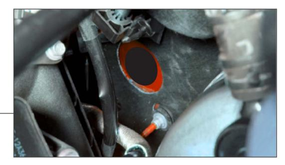
Install the provided grommet into the firewall in place of the sound tube.
