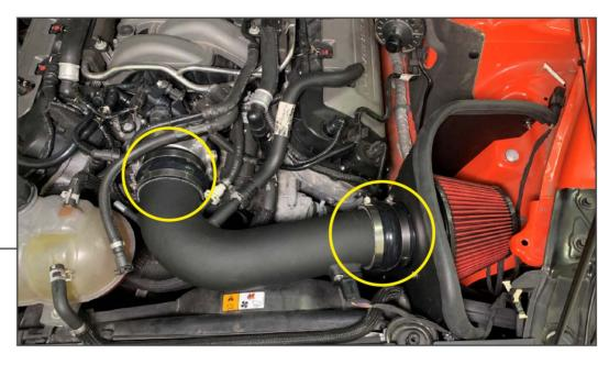
Install the intake tube into the vehicle. Install (1) coupler and (2) hose clamps onto each end of the intake tube. Slide the couplers over the throttle body and the air filter adapter.
