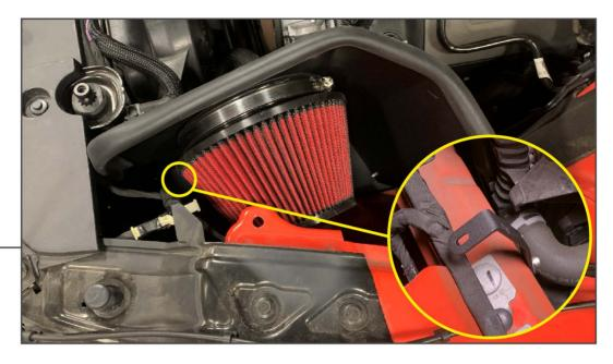
Route the weatherstripping around the edges of the shield, then install the shield and filter into the vehicle. Install (1) M6x1.00 x 20mm bolt, (1) M6 lock washer, and (1) M6 flat washer through the lower bracket and the shield to secure the shield to the vehicle.
