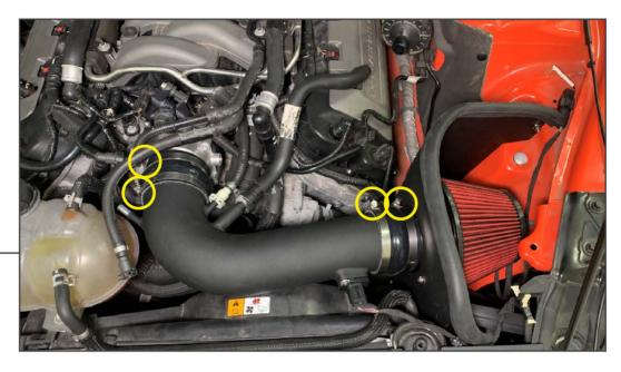
Tighten all of the hose clamps on the intake tube once the intake is fully connected to the vehicle.
