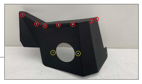
Assemble the (1) large shield and (1) small shield together using (7) M4x0.7 x 8mm Allen bolts and (7) M4 locking nuts. Install the air filter into the shield. Secure the air filter adapter to the air filter using the provided hose clamp. Insert the filter into the shield, then use the provided (2) M6x1.00 x 15mm Allen bolts, (2) M6 lock washers, and (2) M6 flat washers. Tighten all hardware until secure.
