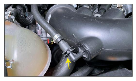
Push in the dark gray portion of the vacuum lines to remove the lines from the intake tube.
