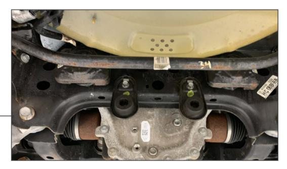
Reinstall the under axle exhaust hangers using the factory hardware.
