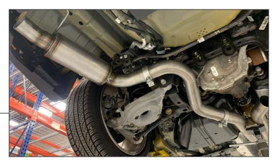
Install the assembled pipe from Step 8 onto the vehicle. First slide an exhaust clamp on the y-pipe than slide the assembled pipe into the exhaust hangers and onto the y-pipe. Repeat this process on both sides.
