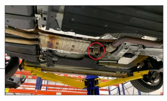
Loosen the (2) 15mm nuts securing the Y-pipe to the downpipe.
