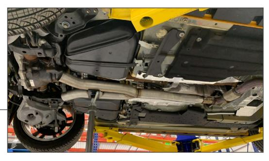
Install the y-pipe so that the flat portion of the exhaust brace is facing down. Use the factory clamp to secure the y-pipe to the downpipe.
