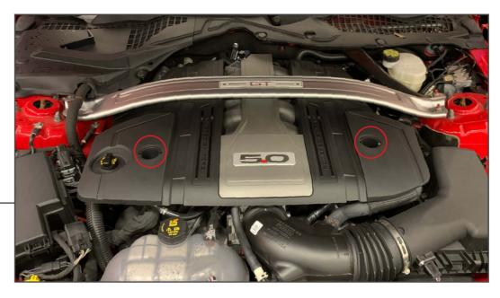
Use a soft pry tool to remove the bolt covers. Then use a 10mm socket to remove the (2) bolts securing the engine cover to the engine. Pull up on the cover and set it aside.
