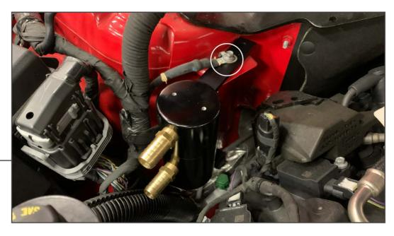
Using the 8mm bolt removed in step 4, mount the oil separator to the vehicle. Ensure the ground cable is install on top of the bracket.
