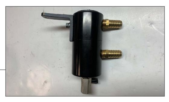
Install the supplied bracket to the oil separator using (1) M6x1.00 14mm bolt, (1) M6 lock washer, (1) M6 flat washer. Install the ball valve on the bottom of the oil separator, use thread sealant to ensure a leak free installation.
