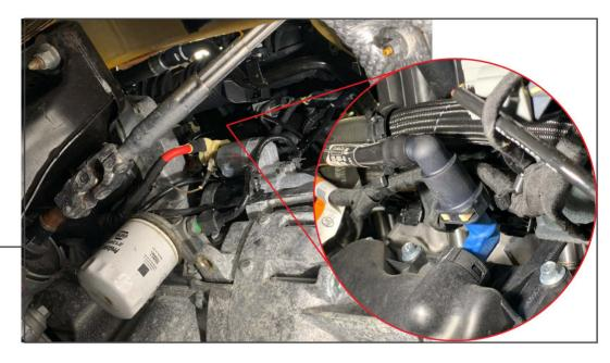
Raise and support the vehicle to gain access to the underside of the intake manifold. Locate the vacuum fitting connected to the side of the engine block. Depress the yellow locking tab and pull it away from the engine.
