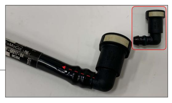
Next, remove the hard-plastic hose from the manifold and valve cover fittings. The fittings have a barb end under the hard-plastic hose. Using a razor blade, carefully cut a relief in the plastic hose and twist the barbed fitting out of the hose. Re-install the fitting onto the intake manifold and valve cover.
