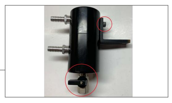
Install the supplied bracket to the oil separator using (1) M6x1.00 14mm bolt, (1) M6 lock washer, (1) M6 flat washer. Install the ball valve on the bottom of the catch can, use thread sealant to ensure a leak free installation.
