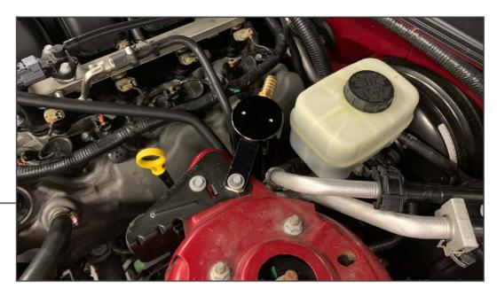
Using the factory bolt, secure the oil separator to the vehicle.
