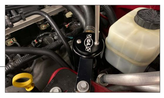
Install the supplied C&L logo plate using (2) M4 Machine screws, and (2) M4 flat washers.
