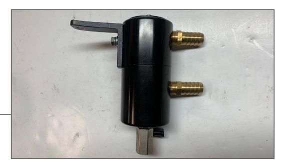
Install the supplied bracket to the oil separator using (1) M6x1.00 14mm bolt, (1) M6 lock washer, (1) M6 flat washer. Install the ball valve on the bottom of the catch can, use thread sealant to ensure a leak free installation.
