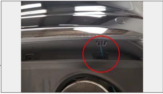
Insert the new MP Concepts light and wiring through the factory diffuser hole making sure the light clips into place. Then using the factory nut from Step 1, secure the light into place.
