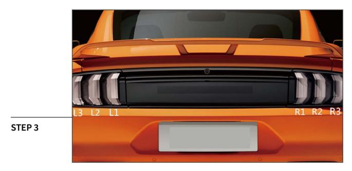
Test fit the covers prior to peeling off the tape backing. Match the small letters on the bottom of each cover to the light position above.
