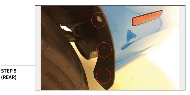
Lift and support the rear of the vehicle. Remove the (3) fasteners securing the outer edge of the fender liner to the bumper cover.
