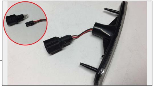
Remove the bulb socket from the original side marker housing. Remove the original light bulb. Plug the new LED marker light into the light socket in place of the light bulb.
