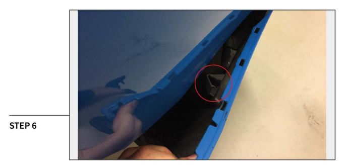
Pull the bumper cover away from the vehicle. Depress the marker light clip to remove the light from the bumper. Unclip the wiring harness from the light.
